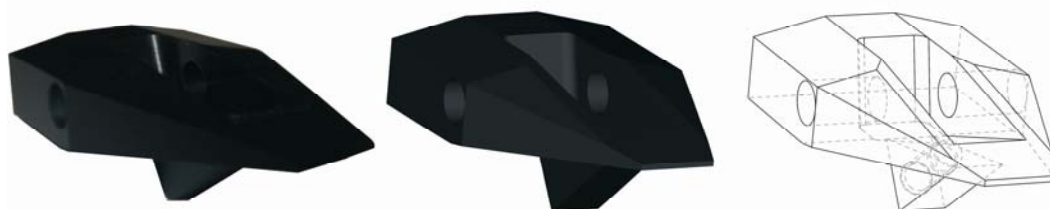
Fig. 2-8 Lower cervical vertebra views: manufacture prototype, 3D model, wireframe
