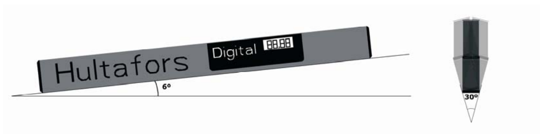
Fig. 3-14 Test performed to the goniometer to know the deviation in the measurements if a rotation of the device is produced
