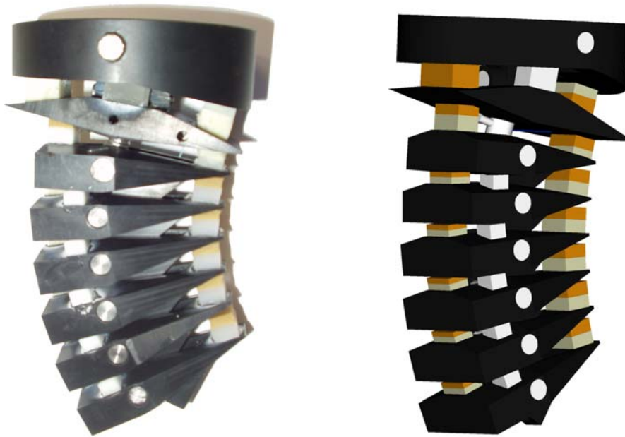
Fig 4-1 Global OmniDirectionalDummy neck II: manufacture prototype and 3D model
