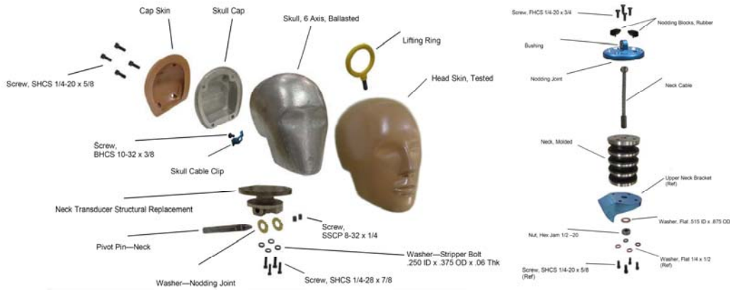
Fig. 1-9 Hybrid III 50 th percentile Head&Neck (adapted from Denton Atd, Inc.)
