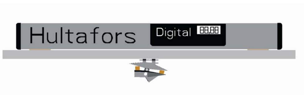
Fig. 3-21 Measurement device for flexion extension between C1C2
