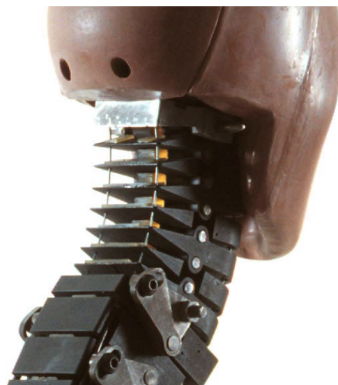
Figure 12: The BioRID-neck (Biofidelic Rear Impact Dummy) has been developed for rear-end collision tests at low velocity.
