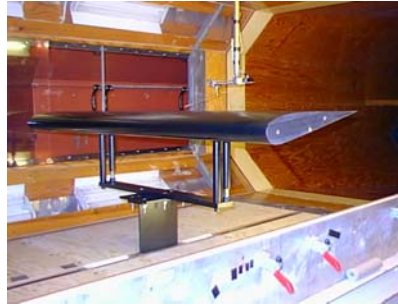
Figure 1. Photo of the airfoil in the wind tunnel
