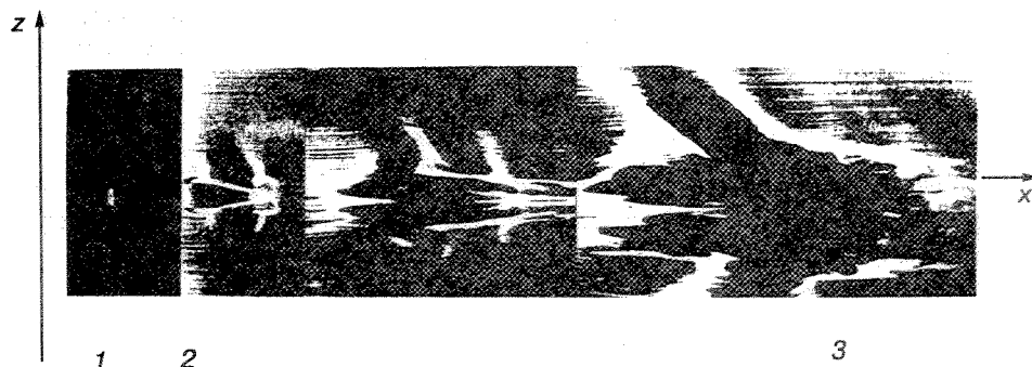
Fig. 2. Visualization picture of \Lambda -structure transformation in a turbulent spot [13]. 1 — a localized disturbance; 2 — \Lambda -vortex; 3 — a turbulent spot; the view in the plane x - z .
