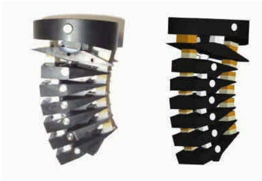
Fig 2.27 Global OmniDirectionalDummy neck II: manufacture prototype and 3D model
