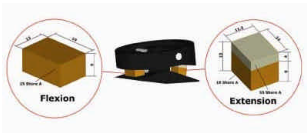
Fig. 2.17 Rubber cushions placed between occiput interface and C1 for flexion/extension
