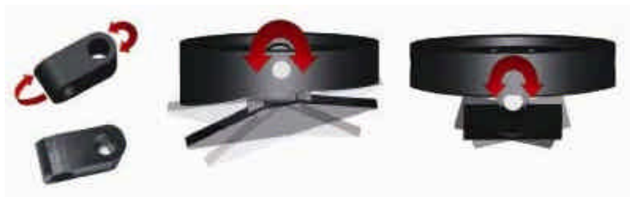
Fig. 2.8 Box views: 3D model, manufacture prototype and possible movements between C0C1: flexion/extension and lateral bending
