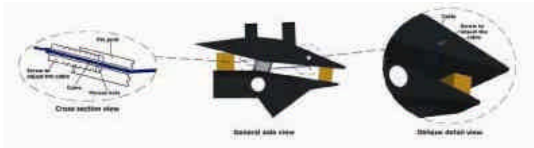
Fig. 2.26 Methods used in the dummy neck to adjust the tension of the cable between C1C2
