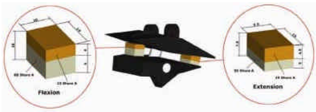
Fig. 2.19 Rubber bumpers located between C1 and C2 vertebrae of the dummy
