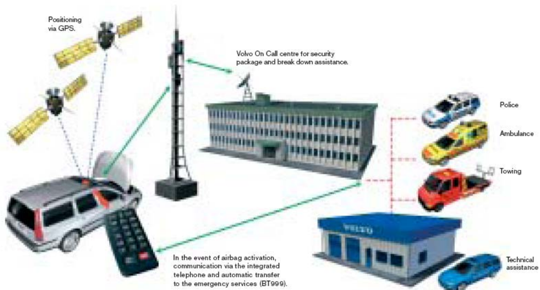
Figure13: Working of Volvo On Call system
